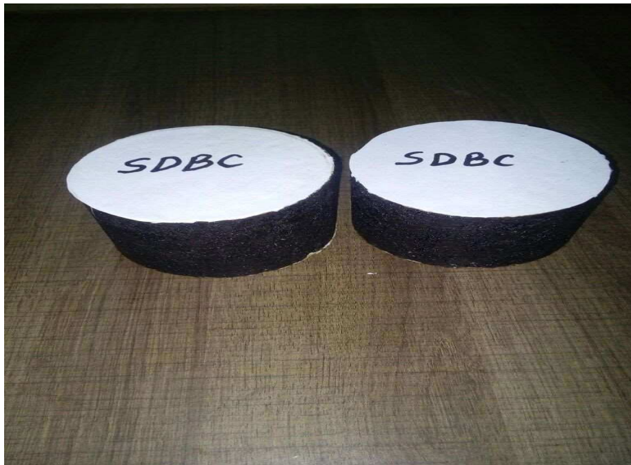
Figure 2: Cold Mix SDBC Marshall Mould
