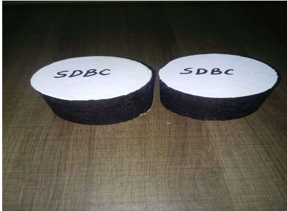
Figure 3: Mould of cold mix SDBC prepared for Marshall test
