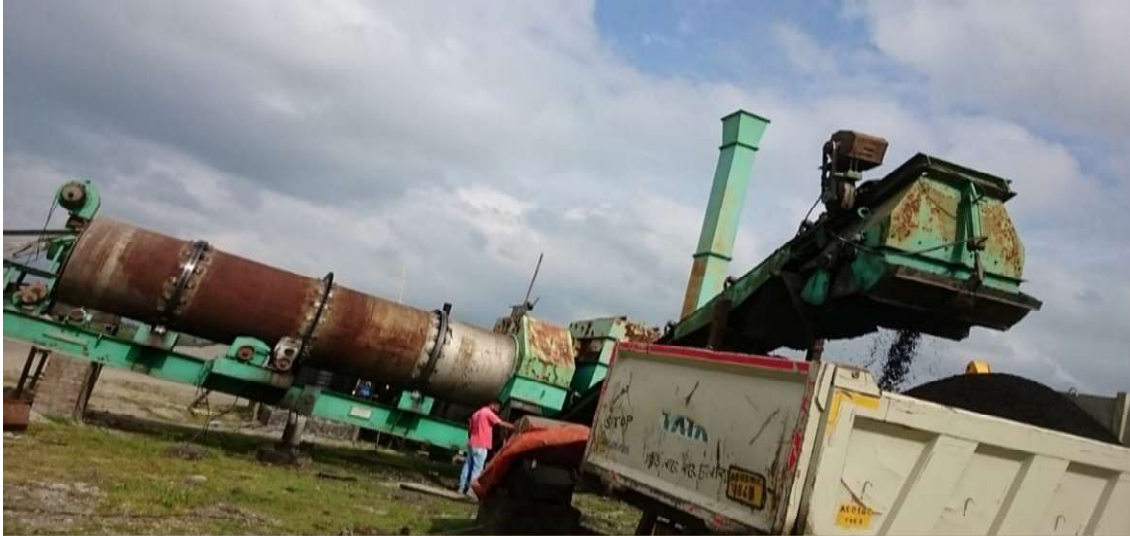
Figure 6: Production of cold mix SDBC through modified HMP
