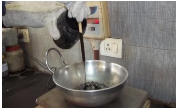
Image – 1, mixing of 10 mm, 6 mm & fines Image – 2, adding cold mix binder as per gradation
