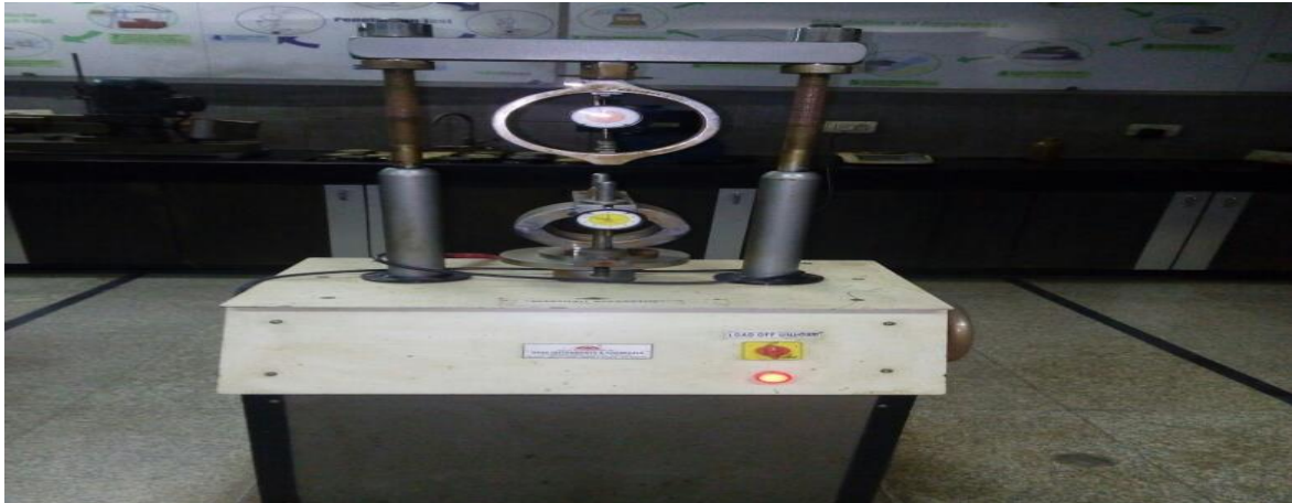
Image – 7, mould of cold mix SDBC prepared for Marshall test
