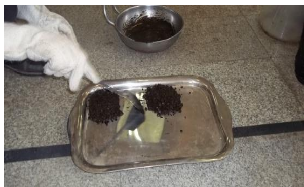
Image-3, preparing cold mix SDBC Image-4, prepared mix is kept on to a tray
