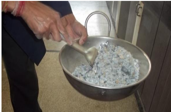
Image – 1, mixing of 10 mm, 6 mm & fines Image – 2, adding cold mix binder as per gradation
