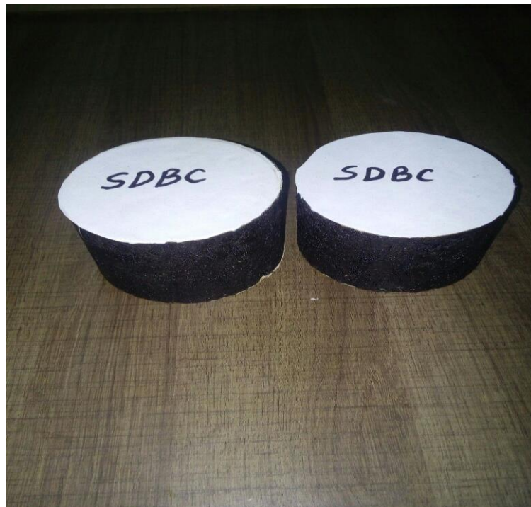
Image – 7, mould of cold mix SDBC prepared for Marshall test
