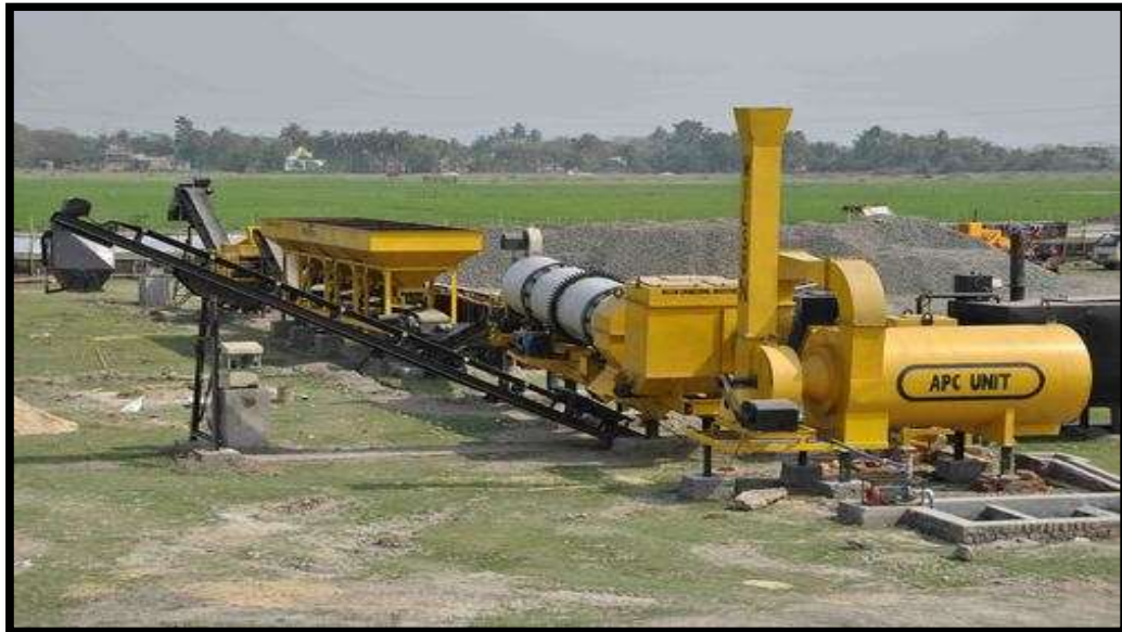
Fig 1: Existing hot mix plant
