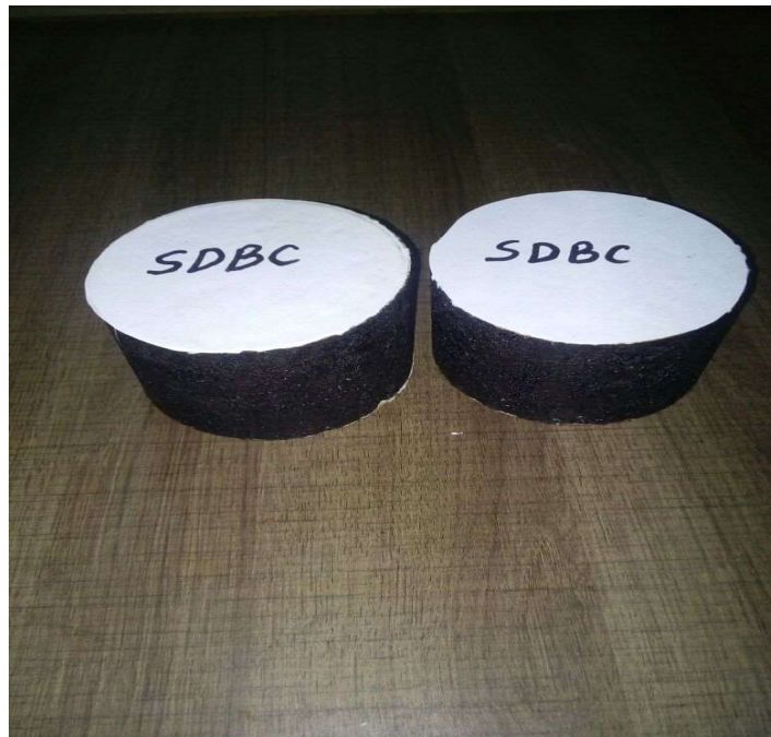
Fig. 7: SDBC mould with 10 mm, 6 mm, fines aggregates and required binder
